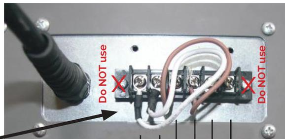
Remove the cover, two screws. Connect the controller as indicated.
